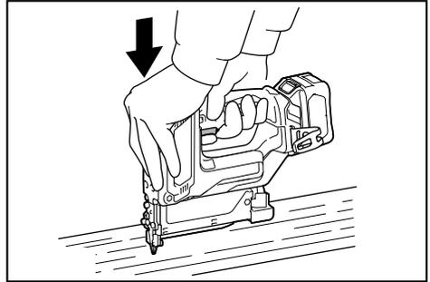
**NOTE:** If the head of the pin nail still remains above the workpiece even you hold the pin nail head, the material may not be suitable for the pin nailer. Continuing to use the pin nailer on such material may result in a damage to the driver of the pin nailer and/or pin nailer jamming.
