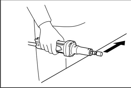
Turn the tool on without the wheel point making any contact with the workpiece and wait until the wheel point attains full speed. Then apply the wheel point to the workpiece gently. To obtain a good finish, move the tool in the leftward direction slowly.
