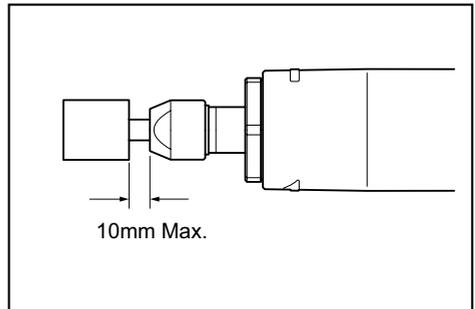
To remove the wheel point, follow the installation procedure in reverse.
