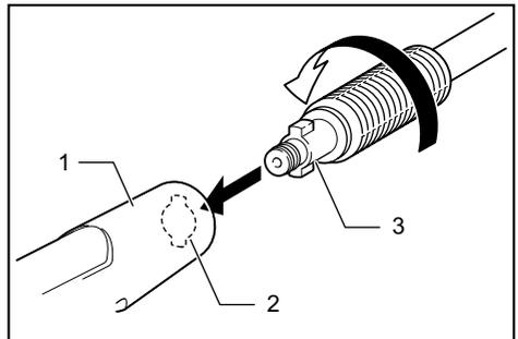
► 1. Trigger gun 2. Slot 3. End of the nozzle
