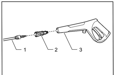
► 1. Nozzle 2. Connecting joint 3. Trigger gun
