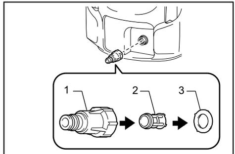
► 1. Water hose connector 2. Filter 3. Sealing ring
