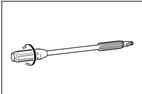
Jet pressure can be adjusted by rotating the nozzle.
