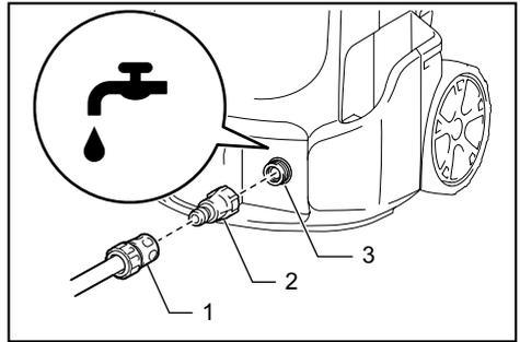
► 1. Coupling sleeve 2. Water hose connector 3. Inlet
