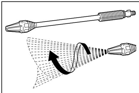
A spiral jet is ejected. Suitable for removing stubborn dirt.
