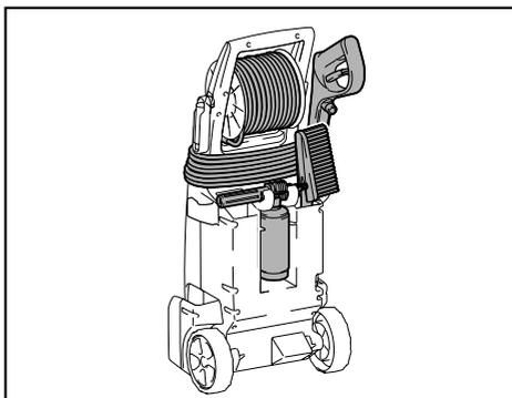
**CAUTION:** Always store in an indoor location where the temperature does not go below freezing. If the high pressure washer freezes and malfunctions, contact your local service center for repairs.
