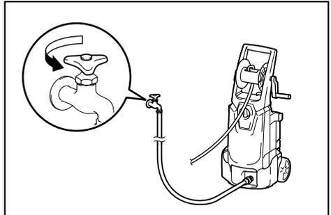
**NOTICE:** To protect the mechanism of the high pressure washer, do not use water hotter than 40°C.
