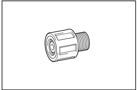
Prevents the high-pressure hose from being twisted.
