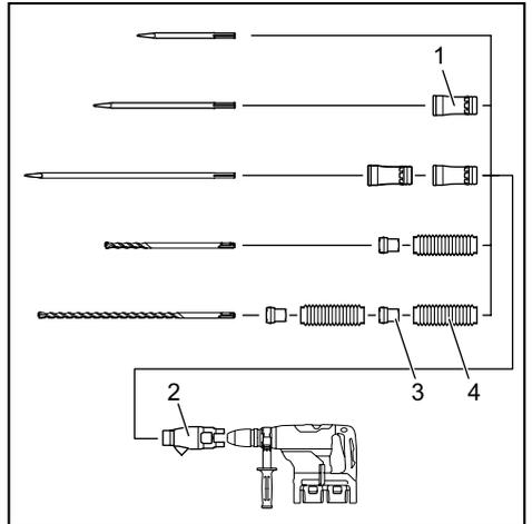
► 1. Dust cover extension 2. Dust cover 3. Joint 4. Bellows
