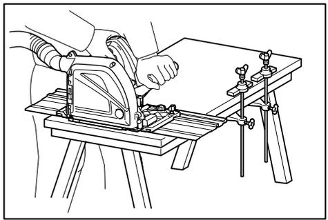
5. **Hold the power tool by insulated gripping surfaces, when performing an operation where the cutting tool may contact hidden wiring or its own cord.** Contact with a "live" wire will also make exposed metal parts of the power tool "live" and could give the operator an electric shock.
