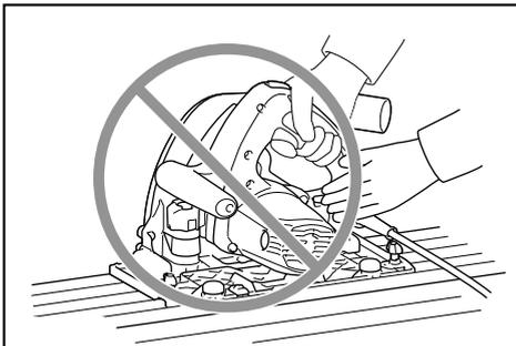
9. **Never force the saw. Push the saw forward at a speed so that the blade cuts without slowing.** Forcing the saw can cause uneven cuts, loss of accuracy, and possible kickback.
