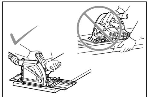
5. Before setting the tool down after completing a cut, be sure that the guard has closed and the blade has come to a complete stop.
