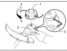
1. Nylon cutting head 2. Spindle 3. Hex wrench
