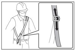
The shoulder harness features a means of quick release.
