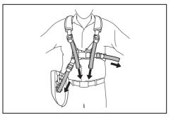
The shoulder harness features a means of quick release.
