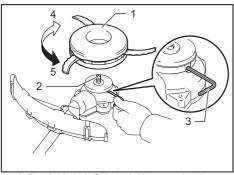
1. Plastic blade 2. Spindle 3. Hex wrench 4. Loosen
