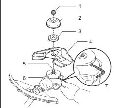
1. Nut 2. Cup 3. Clamp washer 4. Cutter blade
