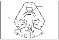
**3.** Put the clamp washer and cup onto the cutter blade and then tighten the nut securely by the box wrench.
