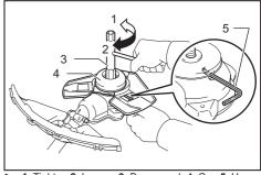
1. Tighten 2. Loosen 3. Box wrench 4. Cup 5. Hex wrench
