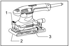
▶ 1. Clamping part 2. Abrasive paper 3. Clamp lever
