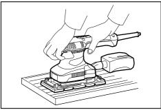
Hold the tool firmly. Turn the tool on and wait until it attains full speed. Then gently place the tool on the workpiece surface. A finishing sander is generally used to remove only a small amount of material at a time. Since the quality of the surface is more important than the amount of stock removed, do not bear down on the tool. Keep the base flush with the workpiece at all times.
