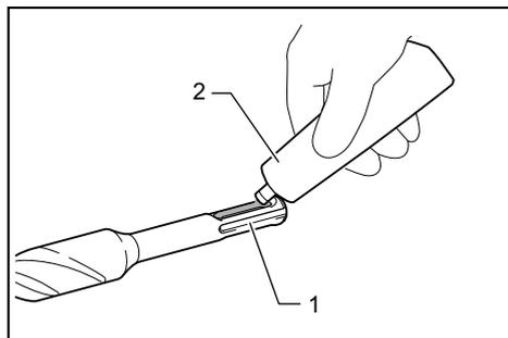
► 1. Shank end of the drill bit/chisel 2. Grease
