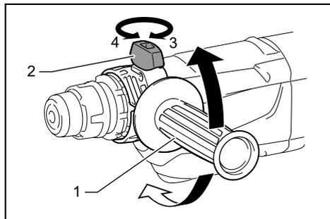
► 1. Side grip 2. Thumb screw 3. Tighten 4. Loosen
