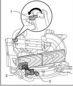
Stopper lever 2. Spacer block 3. Horizontal vise
