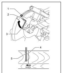
▶ 1. Adjusting screw 2. Range adjustment screw
