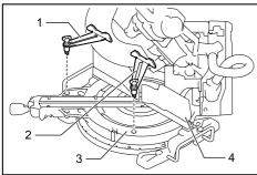
Crown molding stopper L 2. Crown molding stopper R 3. Turn base 4. Guide fence
