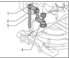
▶ 1. Vise arm 2. Vise rod 3. Clamping screw 4. Vise
