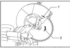
▶ 1. Arrow on the blade case 2. Arrow on the blade
