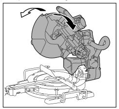
If the pointer does not indicate the 45° position, align it with 45° position by turning the adjusting bolt on the opposite side of the bevel angle scale.
