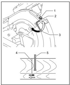
1. Adjusting screw 2. Range adjustment screw
