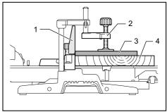
Upper fence 2. Vertical vise 3. Workpiece
