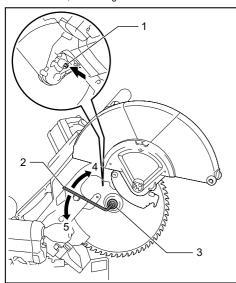
Shaft lock 2. Hex wrench 3. Hex socket bolt (lefthanded) 4. Loosen 5. Tighten
