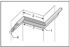
Workpiece 2. Wall width 3. Width of the workpiece 4. Wall contact edge
