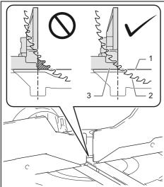
Top surface of turn base 2. Periphery of blade
