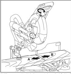
A) When you want to obtain the correct size on the left side of workpiece, shift the laser line to the left of the blade.
