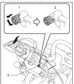
1. Locked position 2. Unlocked position 3. Stopper pin
