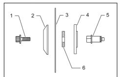
1. Hex socket bolt 2. Outer flange 3. Saw blade
