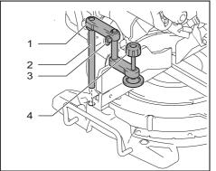
1. Vise arm 2. Vise rod 3. Clamping screw 4. Vise knob
