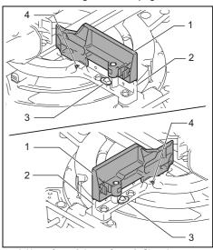
Upper fence 2. Lower fence 3. Clamping screw
