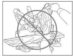
Do not reach behind the fence with either hand closer than 100 mm from either side of the saw blade, to remove wood scraps, or for any other reason while the blade is spinning. The proximity of the spinning saw blade to your hand may not be obvious and you may be seriously injured.
