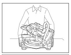
**AWARNING:** Stopper pin for carriage elevation is for carrying and storage purposes only and not for any cutting operations. The use of the stopper pin for cutting operations may cause unexpected movement of the saw blade resulting in kickback and serious personal injury.
