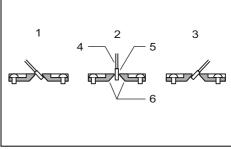
Left bevel cut 2. Straight cut 3. Right bevel cut
