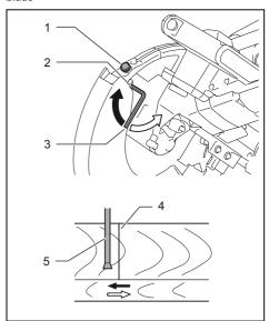
1. Adjusting screw 2. Range adjustment screw
