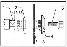
Mounting shaft 2. Inner flange 3. Saw blade
