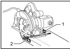
▶ 1. Clamping screw 2. Rip fence (Guide rule)
