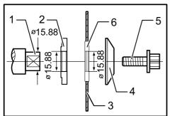
1. Mounting shaft 2. Inner flange 3. Saw blade
