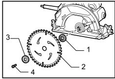
Inner flange 2. Saw blade 3. Outer flange 4. Hex bolt
