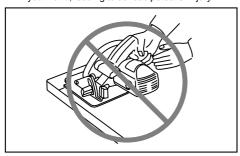
Never force the saw. Push the saw forward at a speed so that the blade cuts without slowing.
