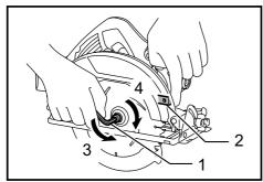
▶ 1. Hex wrench 2. Shaft lock 3. Loosen 4. Tighten
