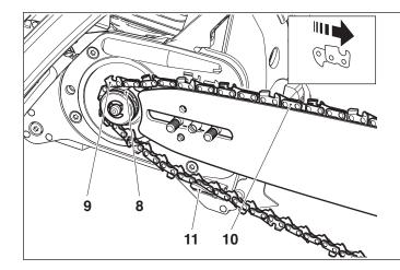
Lift the chain (9) over the sprocket (8).
