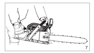
Wrap your fingers tightly around the handles, keeping the handles cradled between your thumb and forefinger (fig. 7). With your hands in this position, you can best oppose and absorb the push, pull and kickback forces of your saw without having it slip out of your grip (see section of reactive forces).
