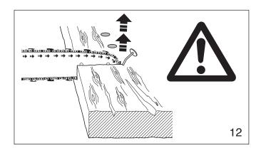
This reaction can occur in a fraction of a second and under some circumstances, cause the guide bar and chain to strike the operator with enough force to cause severe or fatal injury. It may also occur during limbing.
