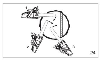
For the sectioning method (fig. 24) make the first cut with the guide bar fanning in toward the hinge. Then, using the bumper spike as a pivot, reposition the saw for the next cut. Avoid repositioning the saw more than necessary.
