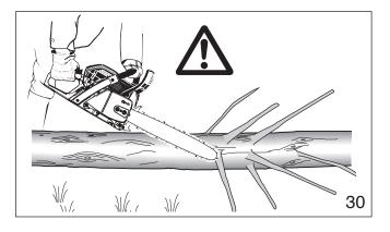
Start limbing by leaving the lower limbs to support the log off the ground (fig. 30). Always cut from the top of the limb.
