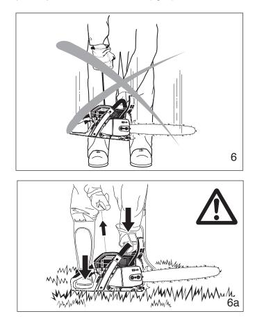
Place the chain saw on firm ground or other solid surface in an open area. Maintain a good balance and secure footing. Place your right foot through the rear handle opening and firmly grasp the front handle with your left hand (fig. 6a).
