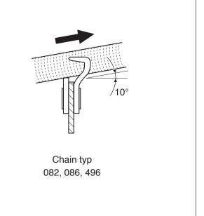
A file holder makes file guidance easier. It is marked for the correct sharpening angle of:
