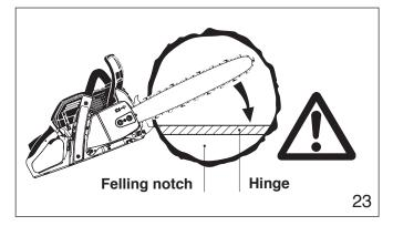
Then, determine the placement of the felling notch (fig. 21). The felling notch when properly placed de-termines the direction in which the tree will fall. It is made perpendicular to the line of fall and should be as close to the ground as possible.
