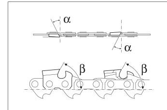
The sharpening angle ( $\alpha$ ) must be identical for all cutters!
