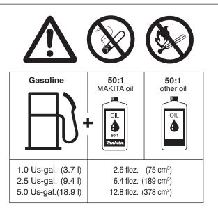
It is not wise to add more engine oil than specified to ensure safe operation. This will only result in a higher production of combustion residues which will pollute the environment and clog the exhaust channel in the cylinder as well as the muffler. In addition, fuel consumption will rise and performance will decrease.
