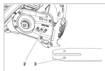
To ensure troublefree operation of the oil pump the oil guide groove at the crank case (2) and the oil inlet bore in the guide bar (3) must be cleaned regularly.
