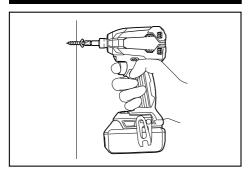
The proper fastening torque may differ depending upon the kind or size of the screw/bolt, the material of the workpiece to be fastened, etc. The relation between fastening torque and fastening time is shown in the figures.
