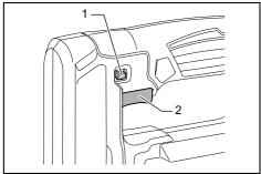
▶ 1. Trigger-lock button 2. Switch trigger
