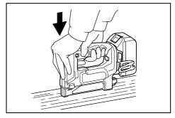
The material may be unsuitable, if the head of driven staple remains above the workpiece surface although the stapler head is held firmly.
