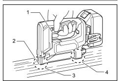
Switch trigger 2. Contact element 3. Front part
