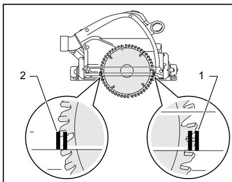
► 1. Front cutting point 2. Rear cutting point
