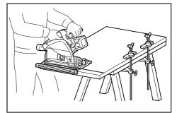
5. Hold the power tool by insulated gripping surfaces, when performing an operation where the cutting tool may contact hidden wiring or its own cord. Contact with a "live" wire will also make exposed metal parts of the power tool "live" and could give the operator an electric shock.
