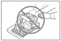
Never force the saw. Push the saw forward at a speed so that the blade cuts without slowing. Forcing the saw can cause uneven cuts, loss of accuracy, and possible kickback.
