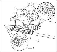
▶ 1. Clamping screw 2. Sub base
