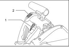
• 1. Switch trigger 2. Lock-off button
