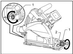
▶ 1. Clamping screw 2. Bevel scale plate
