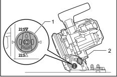
1. Positive stopper 2. Clamping screw
