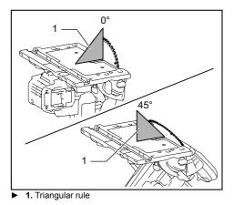
To adjust the 0°-cut accuracy, make the base perpendicular to the blade using a triangular rule, square rule, etc. by turning the adjusting bolt.
