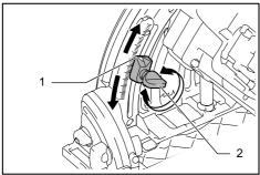
▶ 1. Blade lower limit stopper 2. Clamping screw
