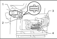
1. Wireless unit 2. Projection 3. Lid 4. Recessed portion When removing the wireless unit, open the lid slowly. The hooks on the back of the lid will lift the wireless unit as you pull up the lid.
