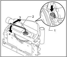
1. Shaft lock 2. Hex wrench 3. Tighten 4. Loosen
