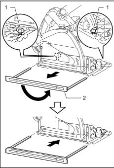
▶ 1. Clamping screw 2. Sub base
