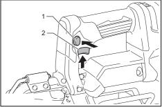
1. Lock-off button 2. Switch trigger
