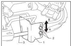
Stopper plate 2. Bolts 3. Band saw blade
