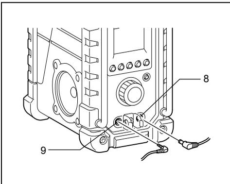
Remove the rubber protector and insert the adaptor plug into the DC socket on the front side of the radio. Plug the adaptor into a standard mains socket outlet. Whenever the adaptor is used, the battery pack is automatically disconnected. The AC adaptor should be disconnected from the main supply when not in use.
