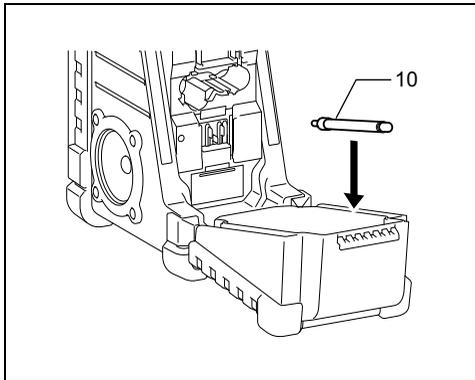
Install the soft bended rod antenna as shown in the figure.
