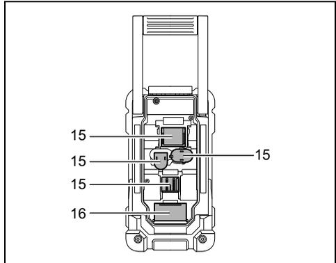
2. Remove back up battery compartment cover and insert 2 fresh UM-3 (AA sizes). Make sure the batteries are with correct polarity as shown inside the compartment. Replace the battery cover.
