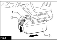
To remove the battery cartridge, slide it from the tool while sliding the button on the front of the cartridge.
