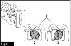
Blade clamp lever 2. Released position 3. Fixed position
