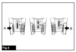
To start the tool, depress the lock/speed change lever from either A or B side and pull the switch trigger. Tool speed is increased by increasing pressure on the switch trigger. Release the switch trigger to stop.
