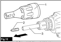
▶ 1. Locator 2. Driver bit 3. Magnetic bit holder
