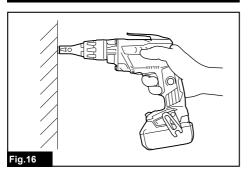
Fit the screw on the point of the bit and place the point of the screw on the surface of the workpiece to be fastened. Apply pressure to the tool and start it. Withdraw the tool as soon as the clutch cuts in. Then release the switch trigger.
