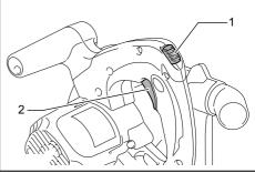
1. Lock-off button 2. Switch trigger
