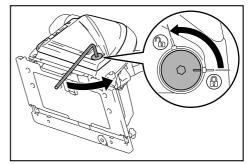
2. Press the shaft lock fully so that the blade does not revolve, then loosen the hex bolt counterclockwise with the wrench.
