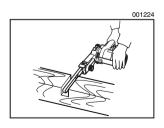
Hold the tool firmly with both hands. Turn the tool on and wait until it attains full speed. Gently apply the tool to the workpiece surface and move the tool forward and back. Press the belt only lightly on the workpiece. Excessive pressure may damage the belt and shorten tool life.
