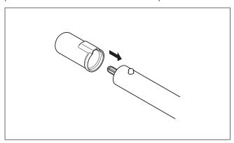
When storing the edger attachment separated from the power unit, put the cap onto the end of the shaft.
