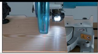
Laser marker and LED joblight for exact cutting
