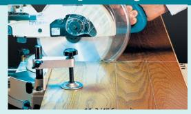
The double sliding mechanism also provides up to 300mm wide cuts at 0° mitre.
