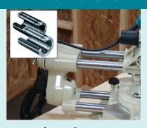
Double sliding mechanism supported by linear ball bearings for accurate/vibration free cuts.
