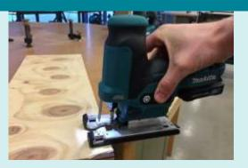
Soft no load - reduces tool vibration and speed when there is no load on the blade
