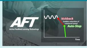
Enhanced safety features including an electric brake, soft-start, and anti-restart
