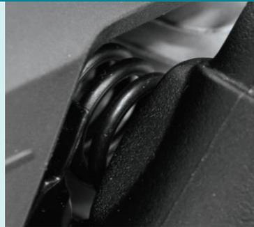
Spring system to minimise vibrations
