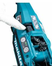
Place in reel and pass wire through hole
