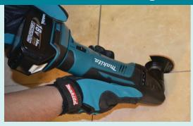
3.2° oscillation angle, accessories can be mounted in 12 positions at 30° intervals
