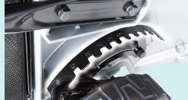
10 stage height adjustment allows the user to select the ideal mowing height
