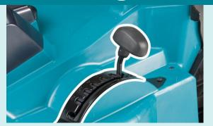
Easy access to height adjustment lever to quickly change settings on the go
