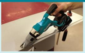
Brushless Motor providing a 3,000spm no load speed
