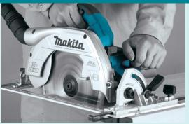
Electric blade brake rapidly slows the blade after trigger has been released
