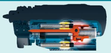
Counter weight mechanism Reduces rebound force
