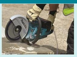
Massive Cutting depth of 88mm
