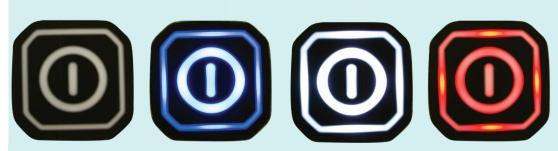
On/off heat controlled with LED indicator Off / Low / Medium / High
