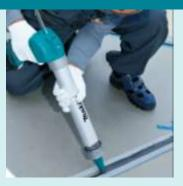
Makita built motor provides 5,000N of dispensing force
